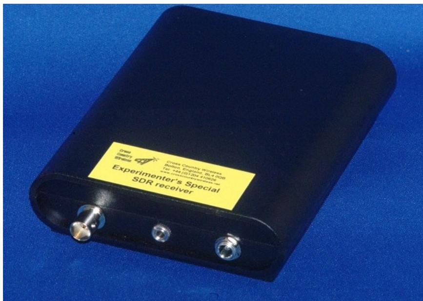
The Experimenter's Special SDR receiver covers 6 to 15 MHz depending on crystals. It has a crystal centre frequency of 7.156 MHz in the X1 crystal position and a HC25/u crystal socket in the X2 position. A selection of crystals are supplied with the receiver covering centre frequencies of 7.056, 9.000 (for some Yaesu, Kenwood and Icom IF frequencies), 10.125 and 14.230 MHz.
