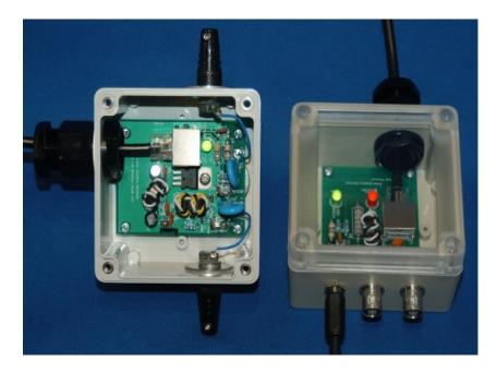
The base unit has two LEDs. The green LED is for DC power indication. The red LED confirms that DC current is flowing to the head unit.
