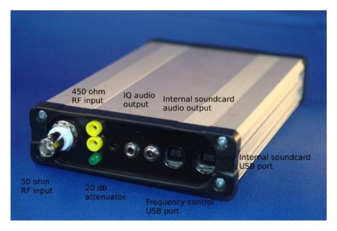
Before starting driver installation remove any external USB hubs from the computer and connect the USB cables from the SDR-4+ receiver directly to the computer USB ports when directed during driver installation. Failure to do this may result in the driver installation being rejected.
