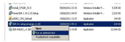
Before starting remove any external USB hubs from the computer and connect the USB cables from the SDR-4+ receiver directly to the computer USB ports when directed during driver installation. Failure to do this may result in the driver installation being rejected.
