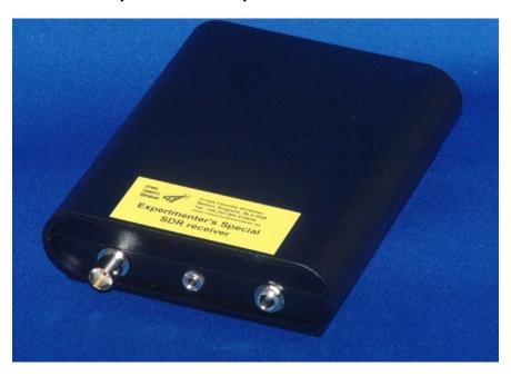
The Experimenter's Special SDR receiver covers 6 to 15 MHz depending on crystals. It has a crystal centre frequency of 7.156 MHz in the X1 crystal position and a HC25/u crystal socket in the X2 position. A selection of crystals are supplied with the receiver covering centre frequencies of 7.056, 9.000 (for some Yaesu, Kenwood and Icom IF frequencies), 10.125 and 14.230 MHz.
